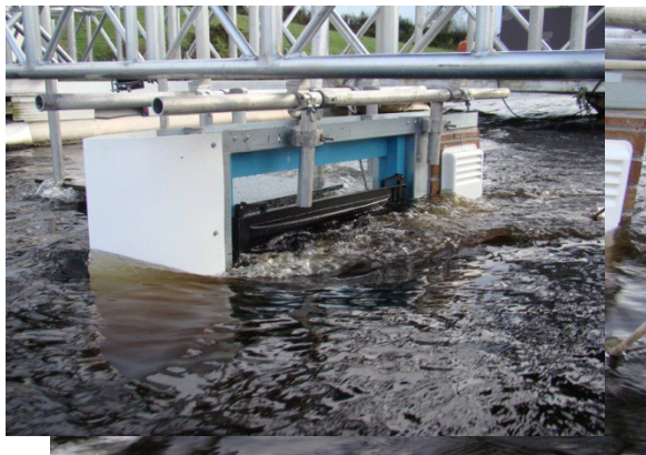
Figure 5, 6 Flooddoor™ in test cell being towed by the catamaran
