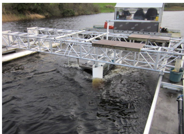
Figure 4 Test cell being towed by catamaran in Montgomery Lake
